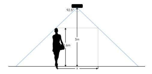
For example, if the Minimum height of pedestrians is 1.6 m, the detection area corresponding to each installation height is as follows:
