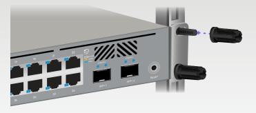
The S8-PoE switch has padding for desktop placement and notches for mounting on the included wall-mount bracket.
