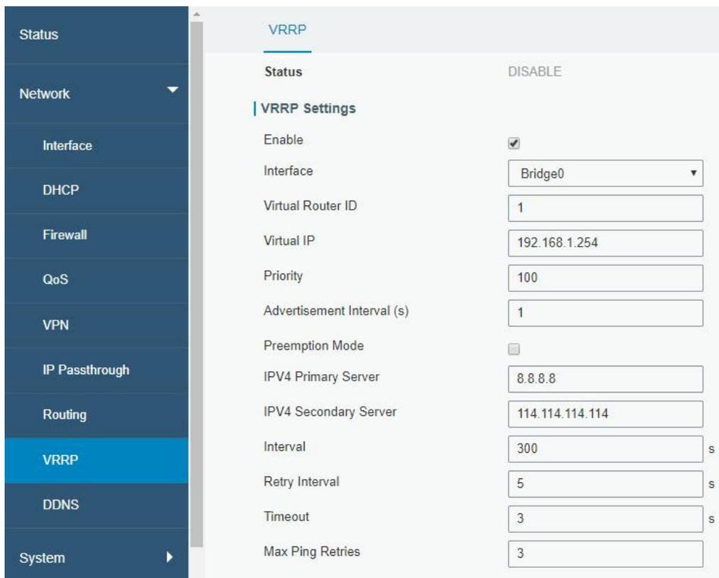
The screenshot shows the VRRP Settings configuration page. The left sidebar contains a menu with the following items: Status, Network (expanded), Interface, DHCP, Firewall, QoS, VPN, IP Passthrough, Routing, VRRP (selected), DDNS, and System. The VRRP Settings section includes the following fields:
