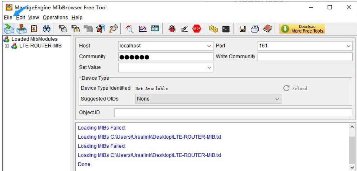
Click the “+” button beside “LTE-ROUTER-MIB”, which is under the “Loaded MibModules” menu, and find “usCellularInfo”. And then you will see the OID of cellular info is “.1.3.6.1.4.1.50234”, which will be filled in the MIB View settings.
