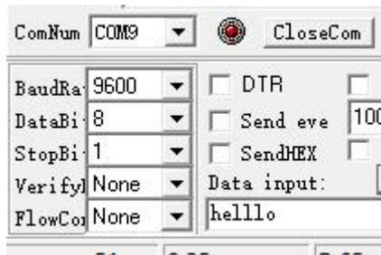
7. After connection is established between the UR32 and the TCP server, you can send data between sscocom and Netassist.
