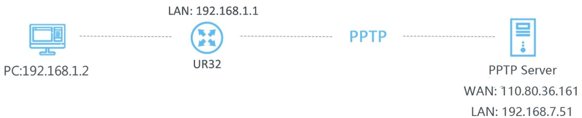
Configure the UR32 as PPTP client to connect to a PPTP server in order to have data transferred securely. Refer to the following topological graph.
