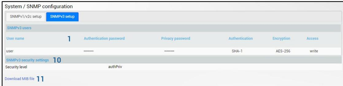
Figure 3-144 SNMP configuration – SNMPv3 setup – status mode
