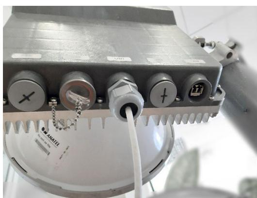
**2** Unscrew the cap of the SFP port (LAN2 or LAN3) that will be used and install an SFP module.
