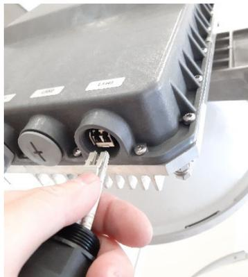
**5** Remove protective covers from the LC connector and connect the connector to SFP module.
