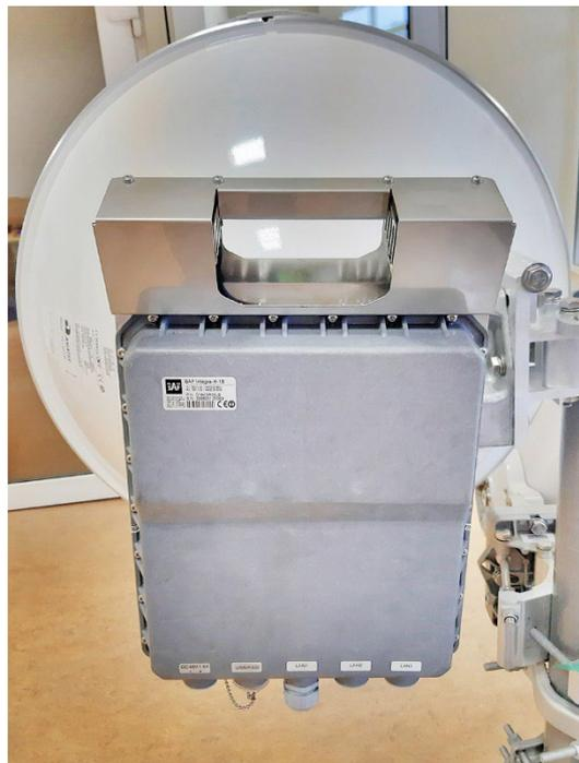
**6** Assembled Integra-E/E2/E3 view. Cables must always be at the bottom of the Integra-E/E2/E3.
