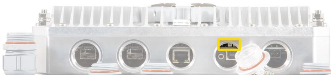
Figure 8-6 RSSI LED placement on FODU
