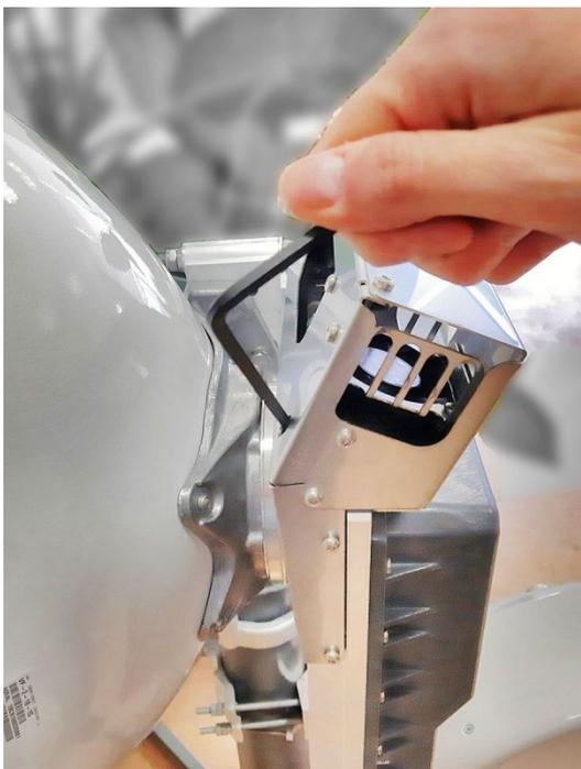
**5** Tighten all four clamp bolts with 3Nm/2.2-foot lbs force.
