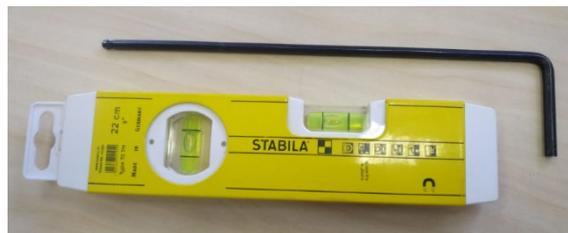
Figure 2-1 Tools for antenna attachment
