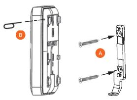
1 Fasten the bracket to the flat surface using the factorysupplied 1.25" x No. 8 mounting screws and plastic wall anchors (A).
